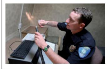
spectrometer that is specifically tuned to measure the intensity of the signals for the C—H bonds in ethanol. For example, the Intoxilyzer 5000 measures the intensity of absorption at the five frequencies illustrated.
