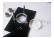
A salt plate used for IR spectroscopy. These plates are moisture sensitive and must be stored in a moisturefree environment.
