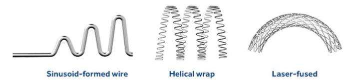
A single strand of cobalt alloy is formed into a sinusoid, wrapped in a helical pattern, and laser fused.
