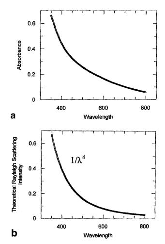
*Figure 1.* (a) Electronic absorbance spectrum of synthetic L-Dopa melanin (20  $\mu$ g/ml in deionized water). (b). Theoretical relationship between Rayleigh light scattering intensity and wavelength.
