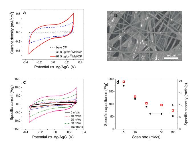
Fig. 1 (a) Cyclic voltammetry of 33.8 μg/cm<sup>2</sup> and 67.5 μg/cm<sup>2</sup> Mel/CP electrodes and bare carbon paper (CP, control sample) in NH<sub>4</sub>CH<sub>3</sub>COO<sub>(aq)</sub> pH 5.5; scan rate 50 mV/s. (b) SEM image, acquired in BSE mode, of a sample made of melanin on carbon paper (CP, loading of ca 0.9 mg/cm<sup>2</sup>) stained with uranyl acetate. The bright areas correspond to melanin chelating the uranyl oxycation.
