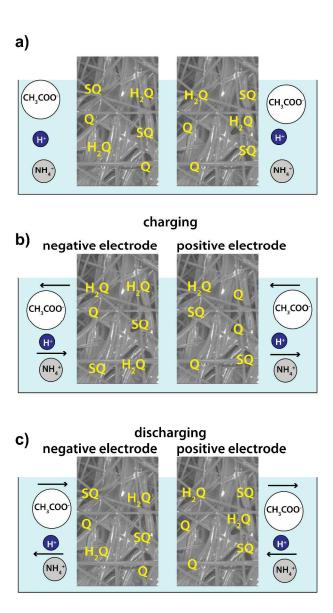
**Fig. 3** Working principle of melanin-based supercapacitors constituted by two identical negative and positive electrodes, immersed in NH<sub>4</sub>CH<sub>3</sub>COOH<sub>(aq)</sub> pH 5.5. a) Situation before a potential is applied between the electrodes, b) situation produced during charging and c) situation produced during the discharging of the electrodes. See Scheme 1 for the chemical structure of H<sub>2</sub>Q, SQ and Q groups.
